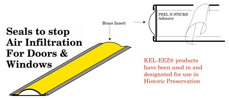
PEEL N STICK Brass seal requires no tacks, nails or screws to install. The seal cuts easily with a large scissors and fastens permanently to wood, metal, composite or coated (painted) surface. The PEEL N STICK® Adhesive has low temperature tack. The bond strength between the weatherstripping and the attaching surface builds with time. Normally you may open the door in about 20 minutes.
